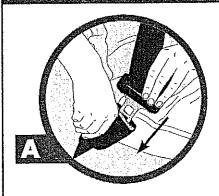
BUCKLE the latch plate into the matching buckle after pulling out the shoulder belt webbing from the seatback. LISTEN for the CLICK sound when the latch plate is fastened!
